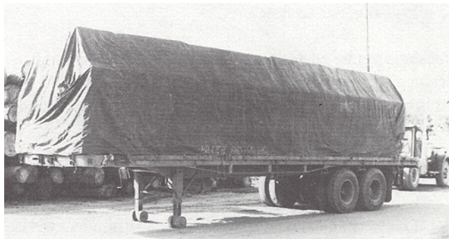
Figure 10-16—Packages of kiln-dried hardwood lumber on a truck trailer are covered with a tarpaulin. (M 142893)
