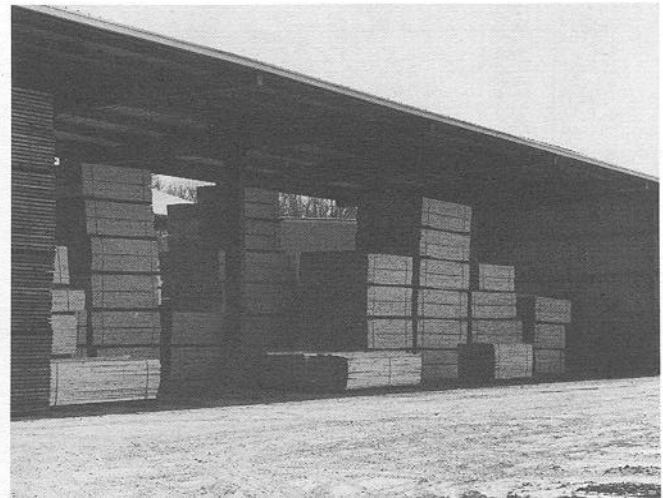
Figure 16-12—Open storage for packages of dry, surfaced lumber. (M88 0164)
